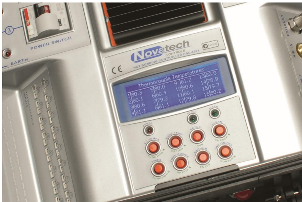
Fig. 22: HBC-4301 Control case keypad and display
